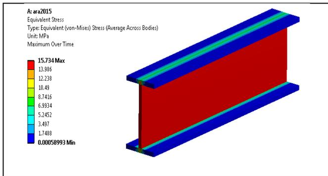
**Fig – 8:** Equivalent Stress of I-Beam with Araldite 2015 Adhesive.
