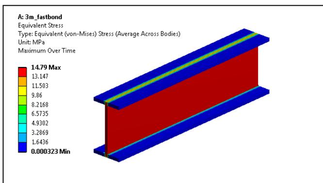
**Fig - 2:** Equivalent Stress of I-Beam with 3M Fastbond Adhesive.
