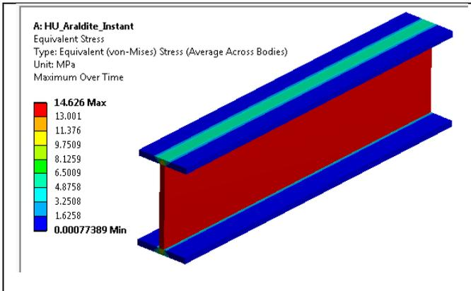
**Fig – 5:** Equivalent Stress of I-Beam with Araldite Instant Adhesive.
