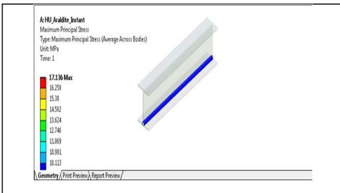
**Fig -6:** Max Principal Stress of I-Beam with Araldite Instant Adhesive.
