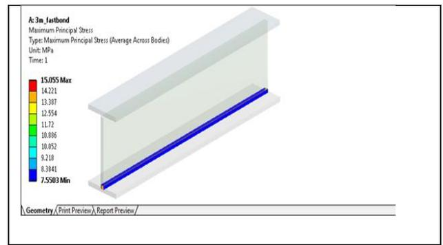
**Fig – 3:** Max Principal Stress of I-Beam with 3M fast bond Adhesive.
