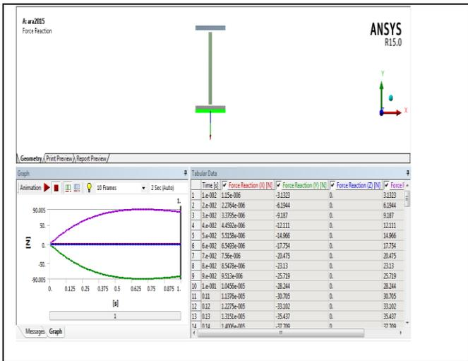
**Fig – 7:** Force Reaction of I-Beam with Araldite 2015 Adhesive.
