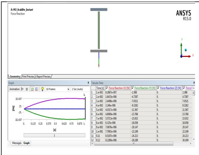
**Fig – 4:** Force Reaction of I-Beam with Araldite Instant Adhesive
