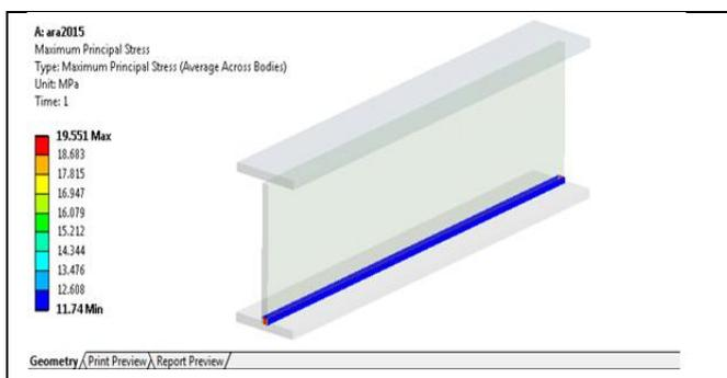
**Fig – 9:** Max Principal Stress of I-Beam with Araldite 2015 Adhesive.
