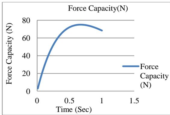
**Chart -1:** Force capacity of I-Beam with 3M Fastbond Adhesive.
